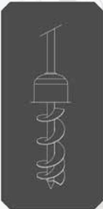
Pole foundation is screwed into place and pole is attached via steel coupling hardware. Special installation equipment is required.
